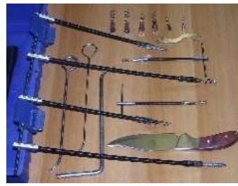
Professional tools for precise cutting under 45°, flexible extractors of used packings, individually or in set
